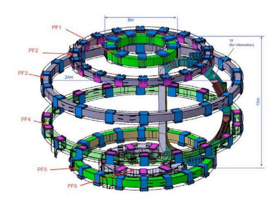
Schematics of the PF Coils Configuration
